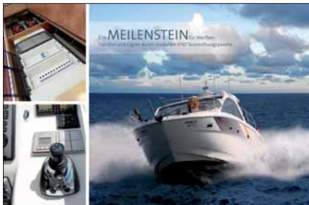
Proficient on the high seas. Stainless steel designer push buttons in the cockpit while the actuator technology is protected in the distribution board in the hull
